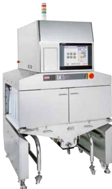
With an inspection chamber height option of 270mm and an X-ray tube voltage of up to 100 kV, the IX-GA-65100 can inspect, for example, a 25kg block of butter, a 65cm-wide case of snack bags or a bag of powdered ingredients. Items can be up to 650mm wide and up to 1000mm in length. The conveyor will run at up to 30m/min and can handle weights of up to 50kg. A version is available (IX-GA-65100-E) which uses a higher resolution X-ray sensor to deliver higher clarity images.
