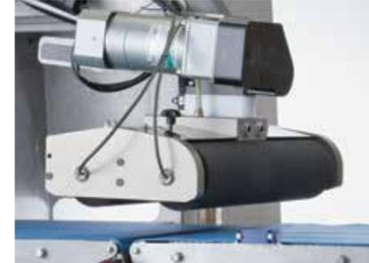
An underside conveyor can be provided with the AirScan platform for sensing around the complete pack.
